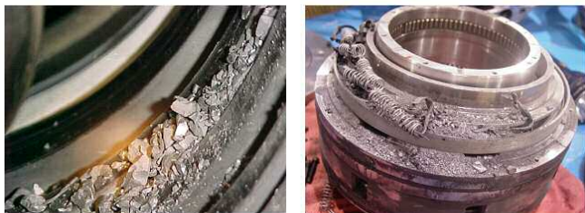
Figure 4. Catastrophic Seal Failure—SiC Fragments that Damage the Seal Head.
