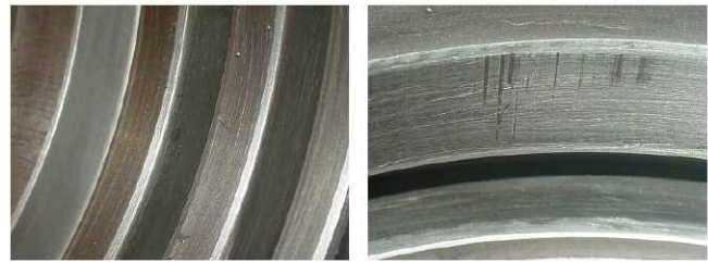
Figure 2. Head Damage at the O-Ring Location Resulting from Rotating SiC Ring Catastrophic Failure.
