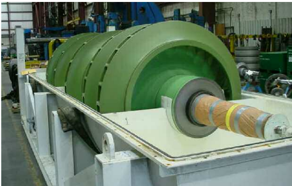
Figure 45. Centrifugal Compressor Rotor Coated with a PTFE Type Coating.
