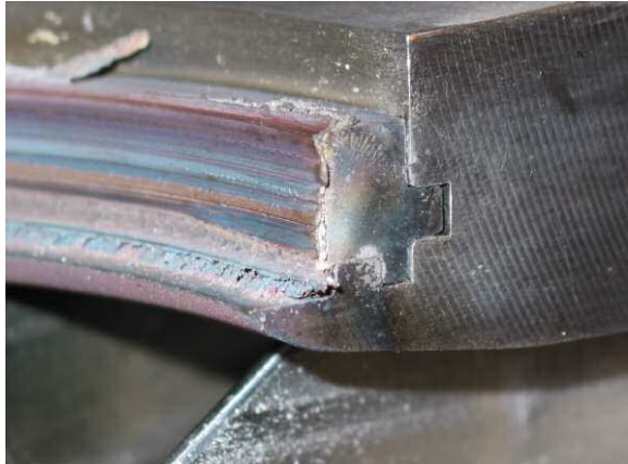
Figure 20. Damage to Nickel Graphite Impeller Seal.
