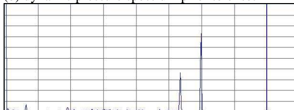
(c) vibration spectrum after onset of impeller stall
