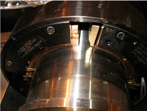
Figure 3. Tilting Pad Journal Pinion Bearing—Evacuated Housing Design.
