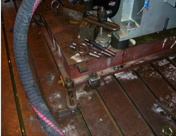
Figure 9. Original Fabricated Hollow Baseplate.
