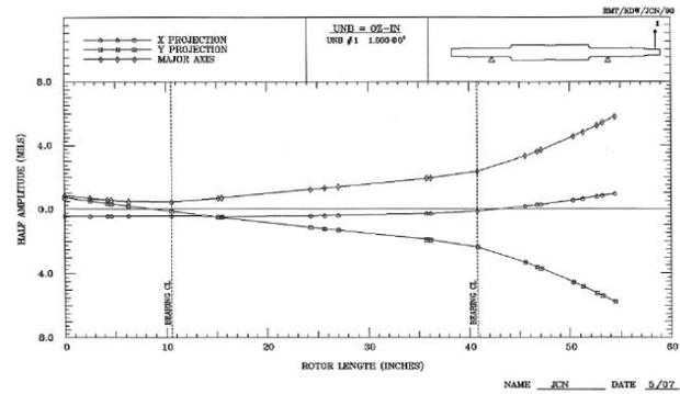
Figure 20. Pinion Mode Shape with Coupling Hub Attachment.
