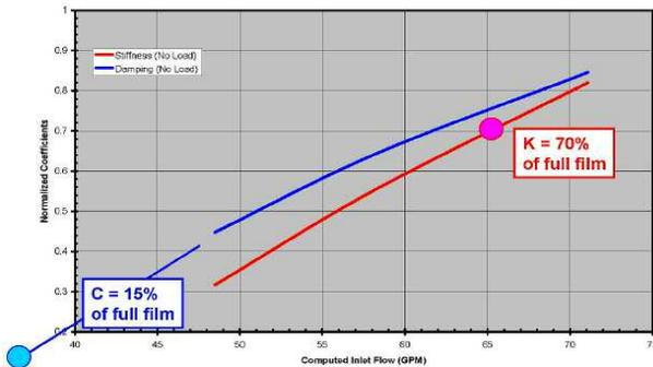
Figure 14. Starvation Model, Normalized  $K$  and  $C$  Versus Oil Flow Showing  $K = 70$  Percent and  $C = 15$  Percent of Full Film Values.
