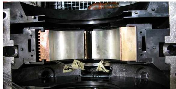
Figure 17. Ultra High Speed Application—Evacuated TPJ Bearing.
