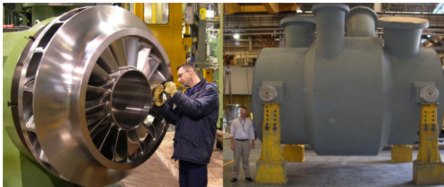
Figure 33. Large LNG Refrigerant Impeller and Mixed Refrigerant Barrel Compressor. (Courtesy General Electric Company)
