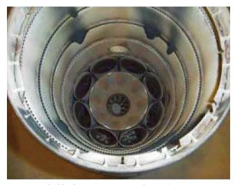
Figure 15 Flashback Damage. (Latcovich, 2002)
