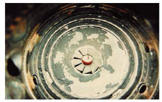
Figure 40. Coked Combustor Nozzle.
