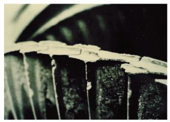
Figure 46. Second Stage Turbine Blade Hot Corrosion Distress.
