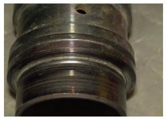
Figure 21. Connecting Tube Damage Due to Pulsations. (Angello and Castaldini, 2004)
