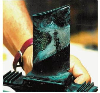
Figure 43. Hot Corrosion Blade Distress.
