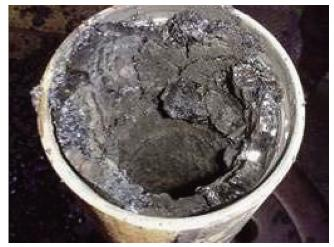
Figure 30. Asphaltene Deposition in an Oilfield Crude Oil Pipeline.
