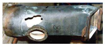
Figure 20. Transition Piece Damage Due to Dynamics.
