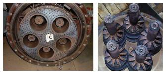
Figure 11. Premix Burner Design (Heavy Duty Gas Turbine).
