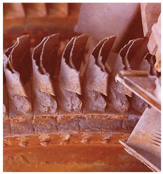
Figure 47. First Stage Blade Damage Due to Liquid Hydrocarbon Related Fire.
