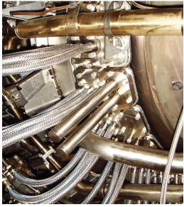
Figure 19. Resonance Tubes in an Aeroderivative Engine (Pulsation Control).
