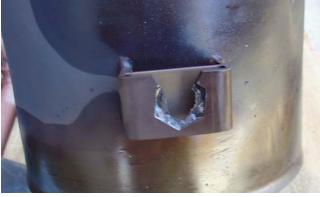
Figure 48. Bracket Damage Due to Vibration and Fretting.
