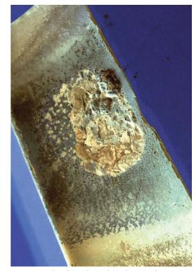
Figure 35. Example of Accelerated Surface Oxidation Caused by Vanadium in Heavy Fuel Oil.
