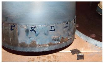
Figure 49. Damage on Liner Seals.
