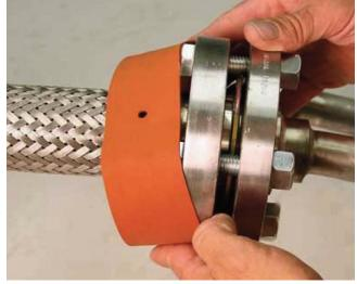
Figure 24. Installation of Band for Flange Leak Testing. (Courtesy Flange Band-It LLC)
