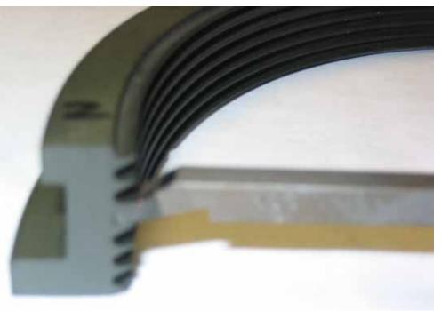
Shaft Seal as removed after 4 and 5 year runs – 9 year total run time – reinstalled will run another 6 years
