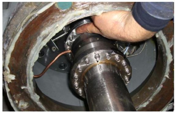
Figure 17. Weight installed on shop test coupling
