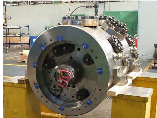
Figure 8. HP compressor casing during hydraulic test
