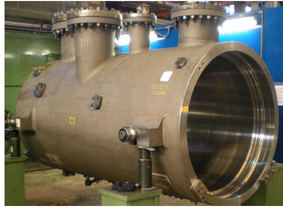
Figure 7. LP compressor casing before hydraulic test
