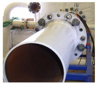
Figure 4: Burst-Membrane Shock-Tube
