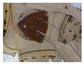
Figure 15: Ariel Reciprocating Compressor with Optical Position Probes Mounted on Valve
