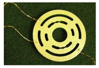
Figure 6: Valve Plate with Reflective Coating and Mounted Strain Gauges
