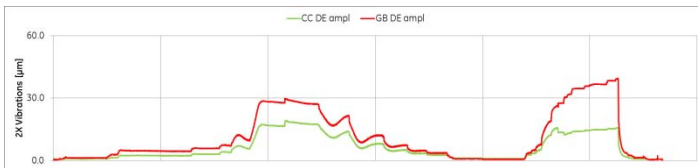
Figure 17: Typical vibration trend recorded on compressor and pinion DE side while oscillating over the resonance frequency
