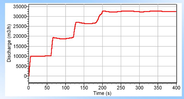
Cooling water flow through condenser at start-up
