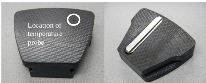
Figure 13: Solid PEEK pad, showing the provision for the fluid film temperature measurement and the metal reinforced pivot.
