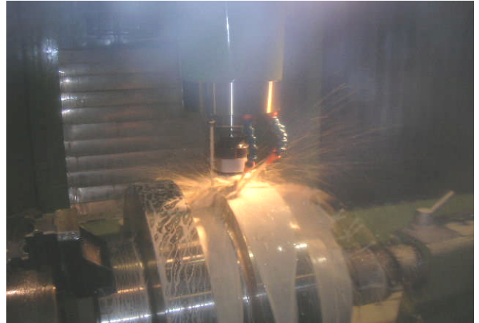
Figure 12: Shaft axial entry dovetail machining qualification
