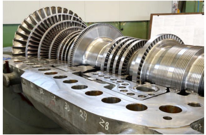
Figure 36: Ethylene charge gas driver turbine
