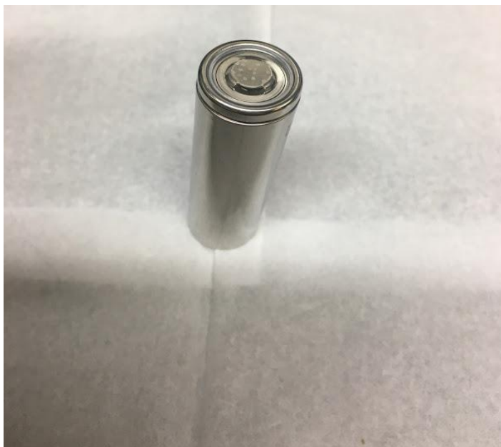
Figure 33 The stainless steel can and the cell header of the cell are exposed after removal of plastic wrapping.
