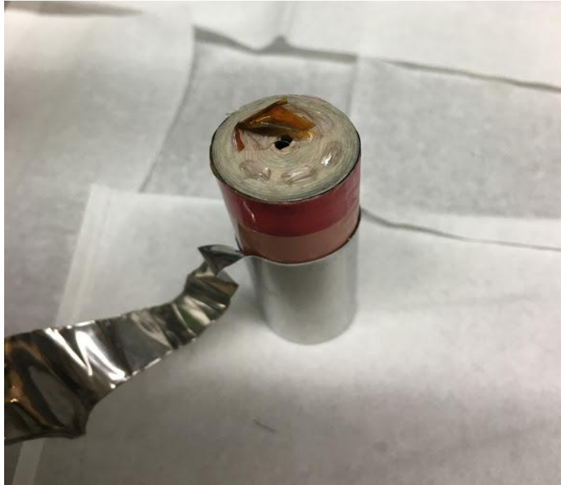
Figure 34 The process of removal of the stainless steel can housing the jelly roll electrodes. Tops of the electrodes, some electrolyte and the cut positive tab are visible.
