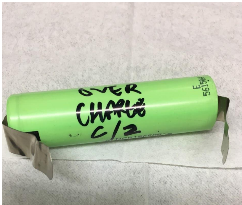
Figure 23 A Panasonic NCR 18650 cell ready to be opened for post-mortem analysis. This cell is placed on a non-metallic surface in order to avoid short circuit of the cell.
