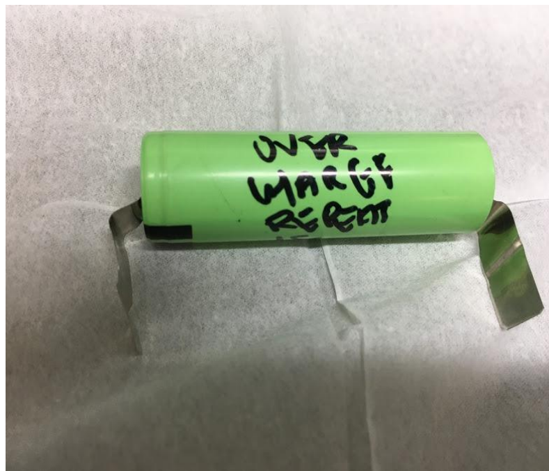
Figure 32 A Panasonic NCR18650B Li-ion cell that has been overcharged and is ready to be disassembled.
