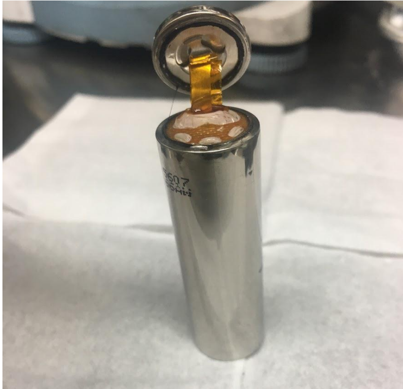
Figure 25 The cell header is cut with a can cutter in order to expose the header and the the main body of the cell. The two parts are connected by the positive tab.
