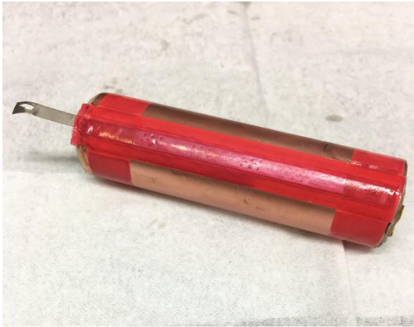
Figure 35 The tape that holds the electrodes together in the jelly roll configuration. A portion of the negative tab that is attached to the anode is visible.
