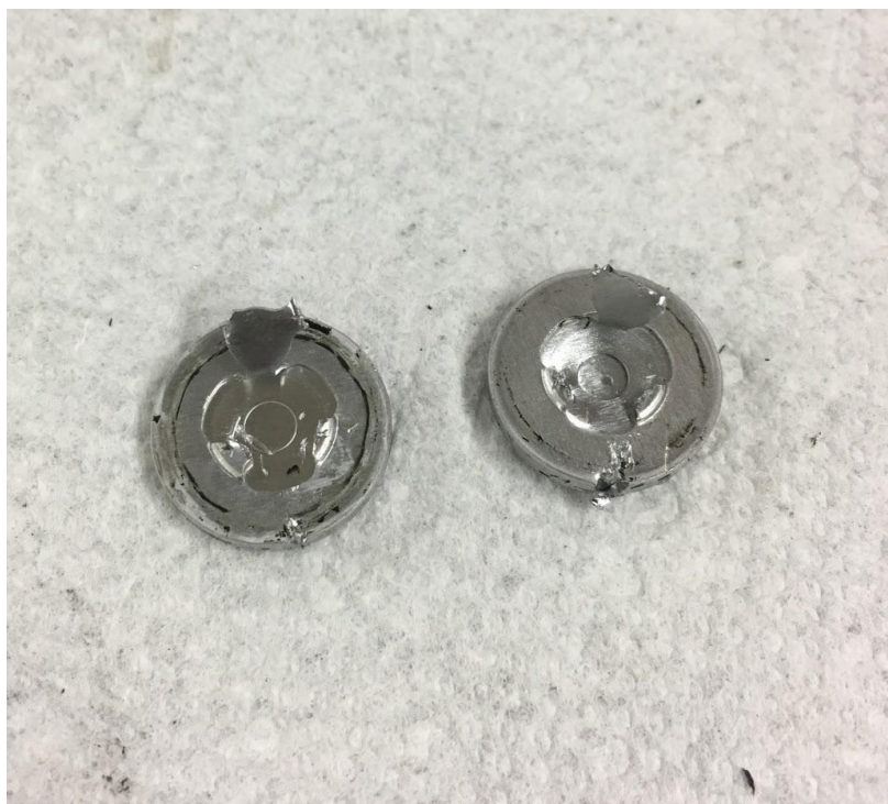
Figure 5 Two current interrupt devices obtained from an overcharged 18650 Li-ion cell.
