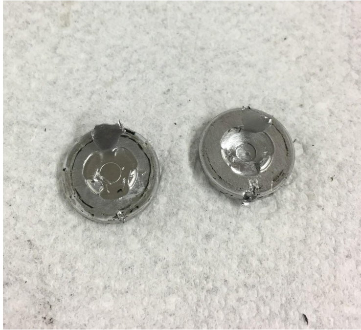
Figure 27 A comparison between an activated and a non-activated current interruption device of a cylindrical Li-ion cell.
