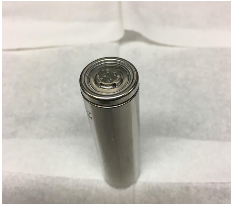
Figure 24 The cell housed in a metal can is visible after removal of the outer plastic layer of the cell.
