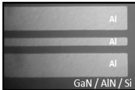
Figure 3-20 Picture of an Al CPW fabricated for GaN-on-Si substrate loss study.
