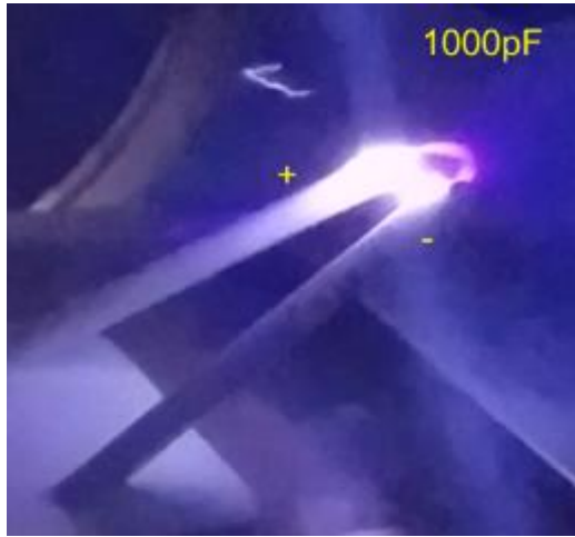
Figure 10. Spark actuator in operation inside SHR tunnel, with C=1000\text{pF} .
