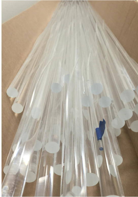
Figure 4.26: Cast PMMA rods produced by PolyOne with attached wire spacers
