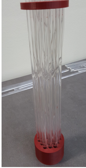
Figure 4.18: 19-rod test assembly
