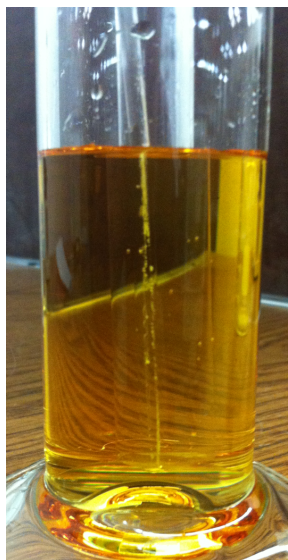
Figure 4.9: PMMA rod and NaI aqueous solution (62 W%) after 1 month of exposure to air at 22°C
