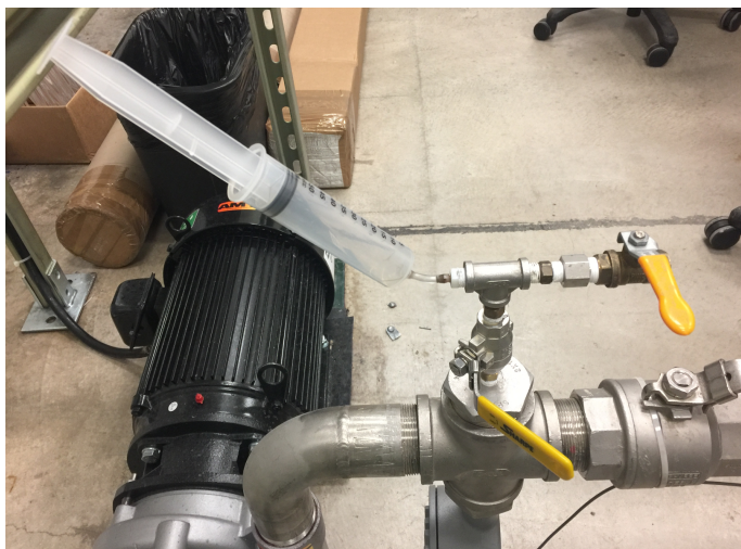
Figure 4.39: Seeding particle injection was performed by manipulating two valves and a 50 mL syringe
