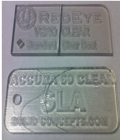
Figure 4.3: VeroClear-RGD810 and Accura 60 samples
