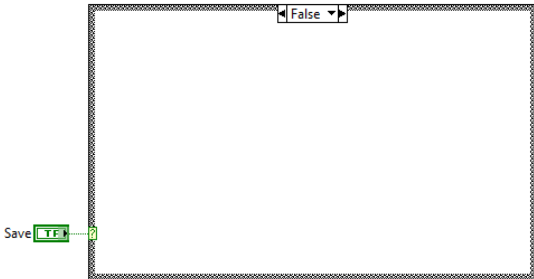
Figure B.62: Save Matrix sub-VI block diagram. If the save command is false, this sub-VI is by-passed.
