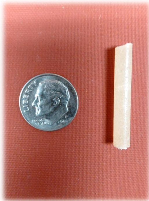
Figure 9: Picture of typical baseline AP/HTPB composite propellant manufactured at Texas A&M University.
