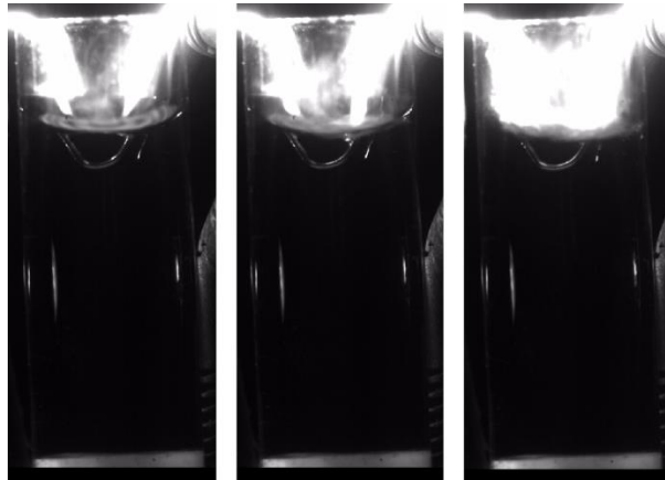
Figure 8 - Frame-by-frame of nitromethane propellant ignition. From left to right, t = -0.0334 , t = -0.0167 , t = 0 seconds.
