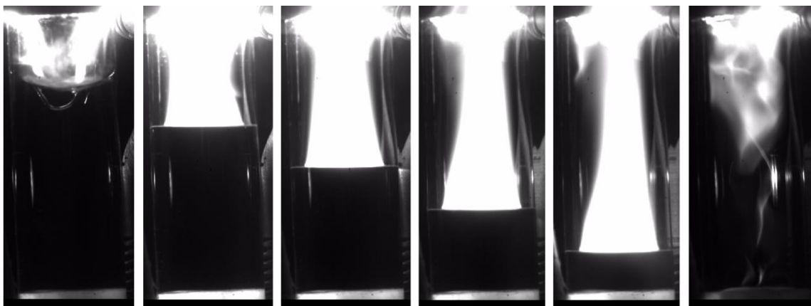
Figure 6 - Images taken from the full nitromethane burn. From left to right, t = 0 , +1.167, +2.334, +3.501, +4.668, and +5.835s.
