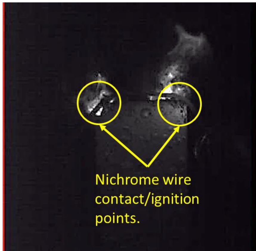
Figure 11 Ignition image using nichrome wire.
