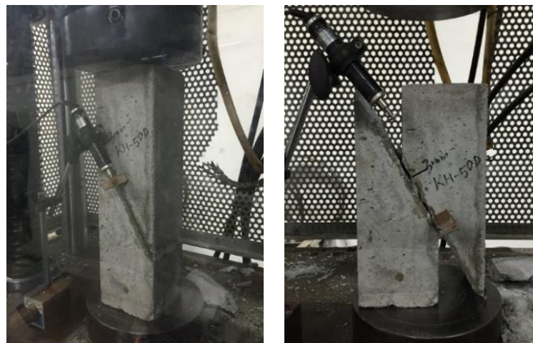
Figure 40 Slant-Shear Test with LVDT Setup
