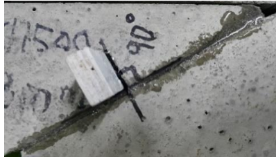
Figure 39 Reference Bar for Measuring the Transverse Displacement
