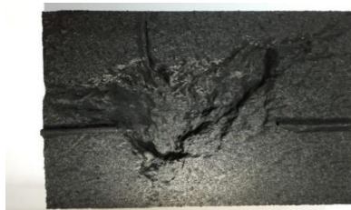
Figure 14 3D Printed Mold for a Concrete Segment
