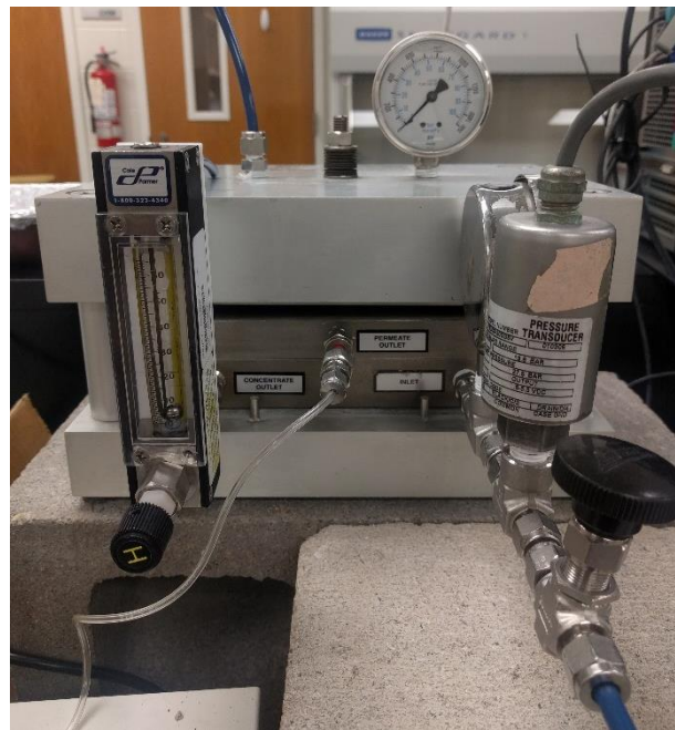
Figure A-13. Stainless-steel plate-and-frame NF/RO cell
