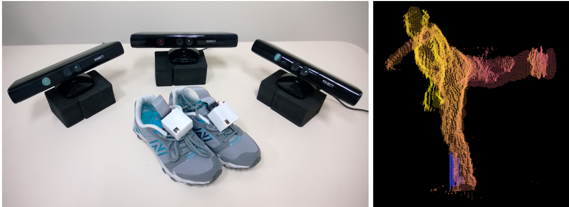
Figure II.4: Data acquisition. (left) three Kinect cameras and a pair of pressure-sensing shoes; (right) input data to our motion capture system includes the point cloud obtained by three cameras and pressure data (blue lines) recorded by pressure sensors.
