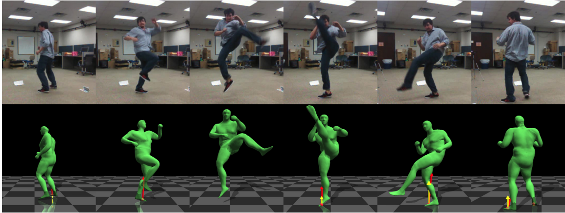
Figure I.1: Our system automatically and accurately reconstructs full-body kinematic and dynamic data using input data captured by three depth cameras and a pair of pressure-sensing shoes. (top) reference image data; (bottom) the reconstructed full-body poses and contact forces (red arrows) and torsional torques (yellow arrows) applied at the center of pressure.
