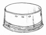
Cut a few holes in the other side a little higher than the opening. This will give the ventilation needed to cause a draft.
