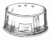
Cut out the bottom of the tub. Cut an opening in one side.
