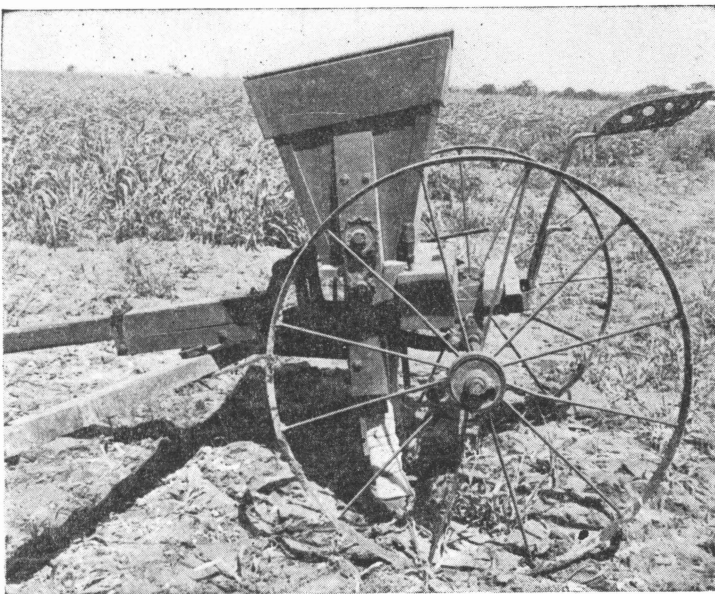
Fig. 1. View of distributor showing picker wheel drive. Handle at driver's feet is to operate in-and-out-of gear mechanism.
