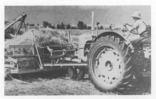
This tractor mounted sweep rake is raised and lowered by a system of levers. (Courtesy of PHILFARMER)
