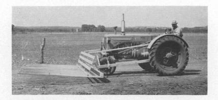
This buck rake is raised by means of the tractor power lift. It may also be used for moving bundle feed. (Courtesy of Capper's Farmer)
