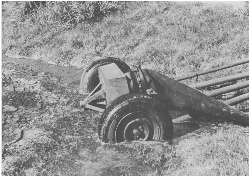
Fig. 4. Lagoon sludge can be removed periodically using trailer-mounted centrifugal pumps, vacuum-loaded tank wagons or other devices.
