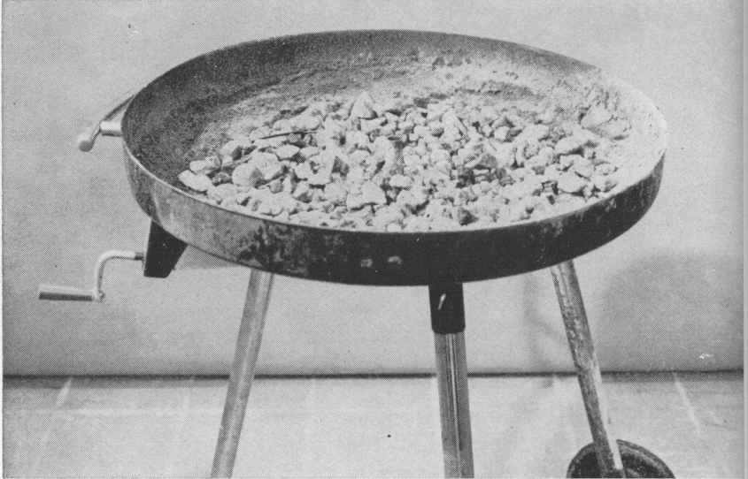
Figure 7.—Place gravel or ceramic material in bottom of fire box.
