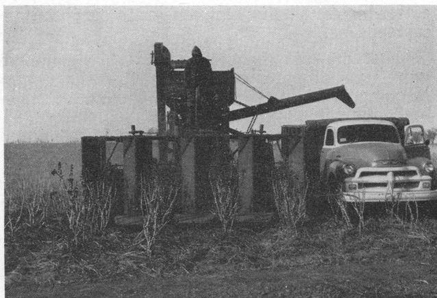
Figure 3. Castorbeans are harvested mechanically with multi-row equipment. A 4-row harvester mounted on a self-propelled combine in use on the High Plains.
