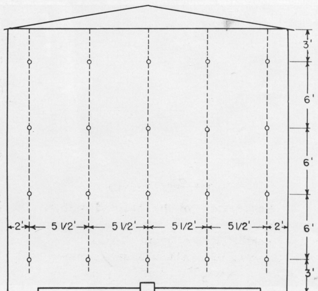
Figure 2. Five cables with thermocouples located at 3, 9, 15 and 21-foot depths were used to determine temperatures at regular intervals during the storage period.
