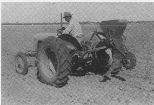
Figure 2. Deep-Feeder fertilizer distributor mounted on a tractor.
