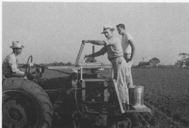
Figure 1. Experimental fertilizer distributor mounted on a tractor.
