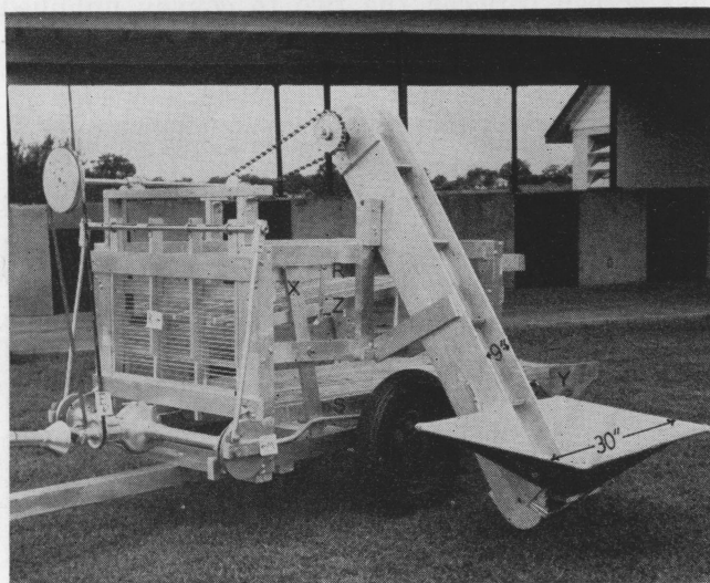
Figure 3. Showing separator-huller ready for operation. R, top screen; Z, middle screen; S, bottom screen; circumference of belt, E, 114 inches; length of pivot bar, X, 33 inches.
