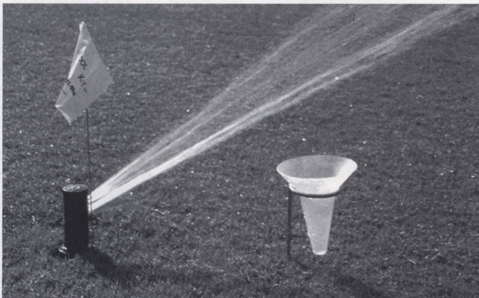
Place the catch can far enough away from the sprinkler head to avoid obstructing the spray pattern.
