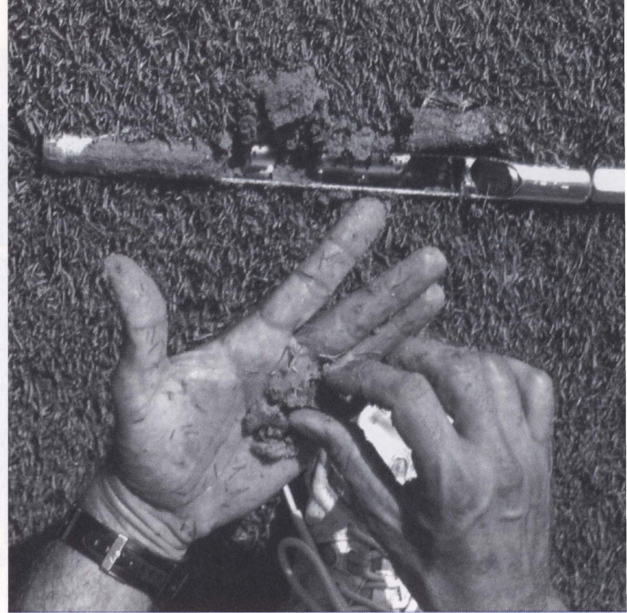
Determine the soil type by feeling soil in the palm of your hand.
