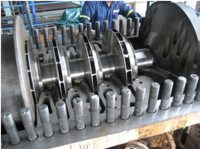
Photo 3: Compressor with non-metallic seals at impeller mouth rings. (appear in white colour)
