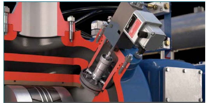
Photo 5: Actuator mounted on a suction valve of typical reciprocating compressor cylinder for achieving stepless control (Image courtesy : Hoerbiger )
