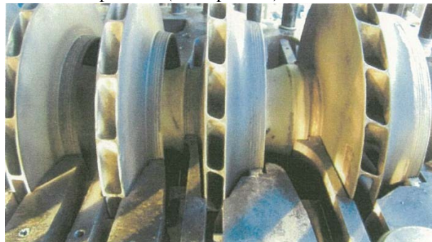
Photo 2: Same Wet Gas compressor rotor condition after close to five years of service.
