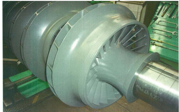
Photo 1: Wet Gas Compressor rotor with coating
