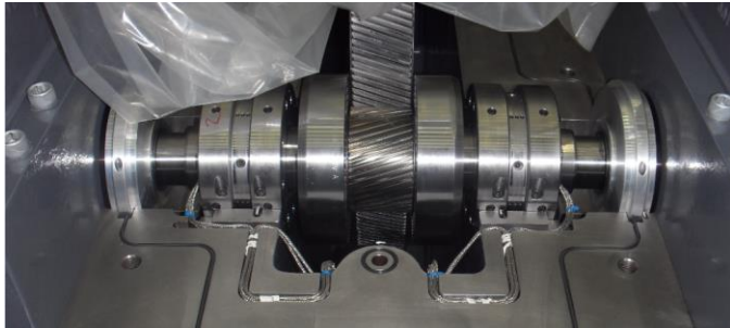
Figure 26. Pinion with Thrust Collar Arrangement
