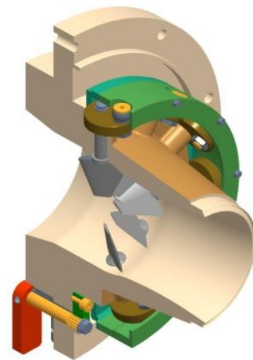
Figure 16. IGV Mechanism to Control Flow Entering
