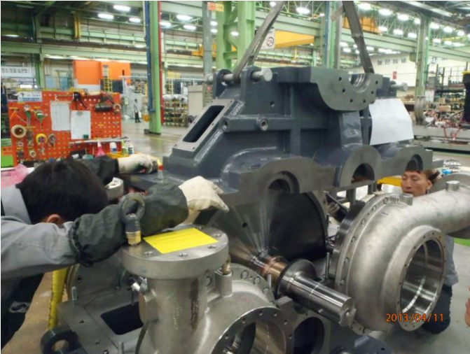
Figure 22. Three Pinion Gear Box, with Mid-section Being Lowered In Place.
