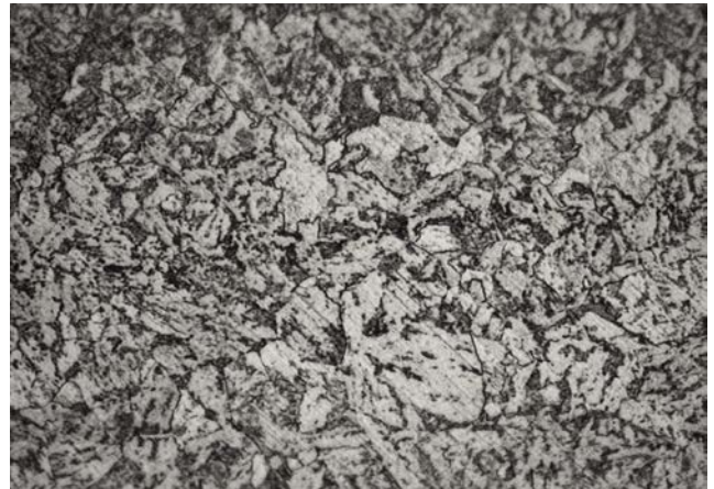
Figure 35. Metallographic Replica, on the Downstream Face of the Last Stage Disk, Showing Less Degradation When Compared to the High Temperature Locations. Etched in 5% Nital. 200X
