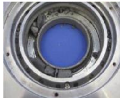
Figure 21: Destroyed seal faces after startup with contaminated sliding faces
