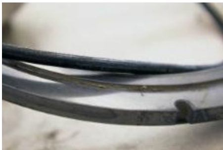
Figure 10: contaminated dynamic sealing element
