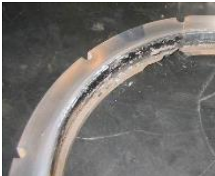
Figure 12: damaged seal faces → damage seal
