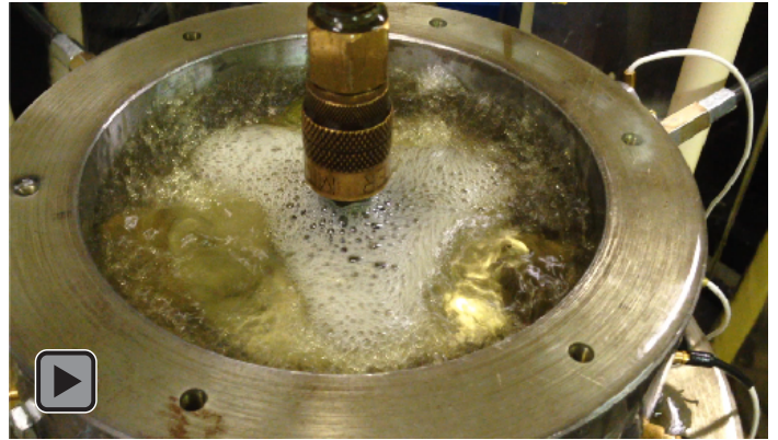
Fig 8. Video depicting outlet foamy lubricant in an open ends SFDs. http://youtu.be/8wQITnGTmyE
