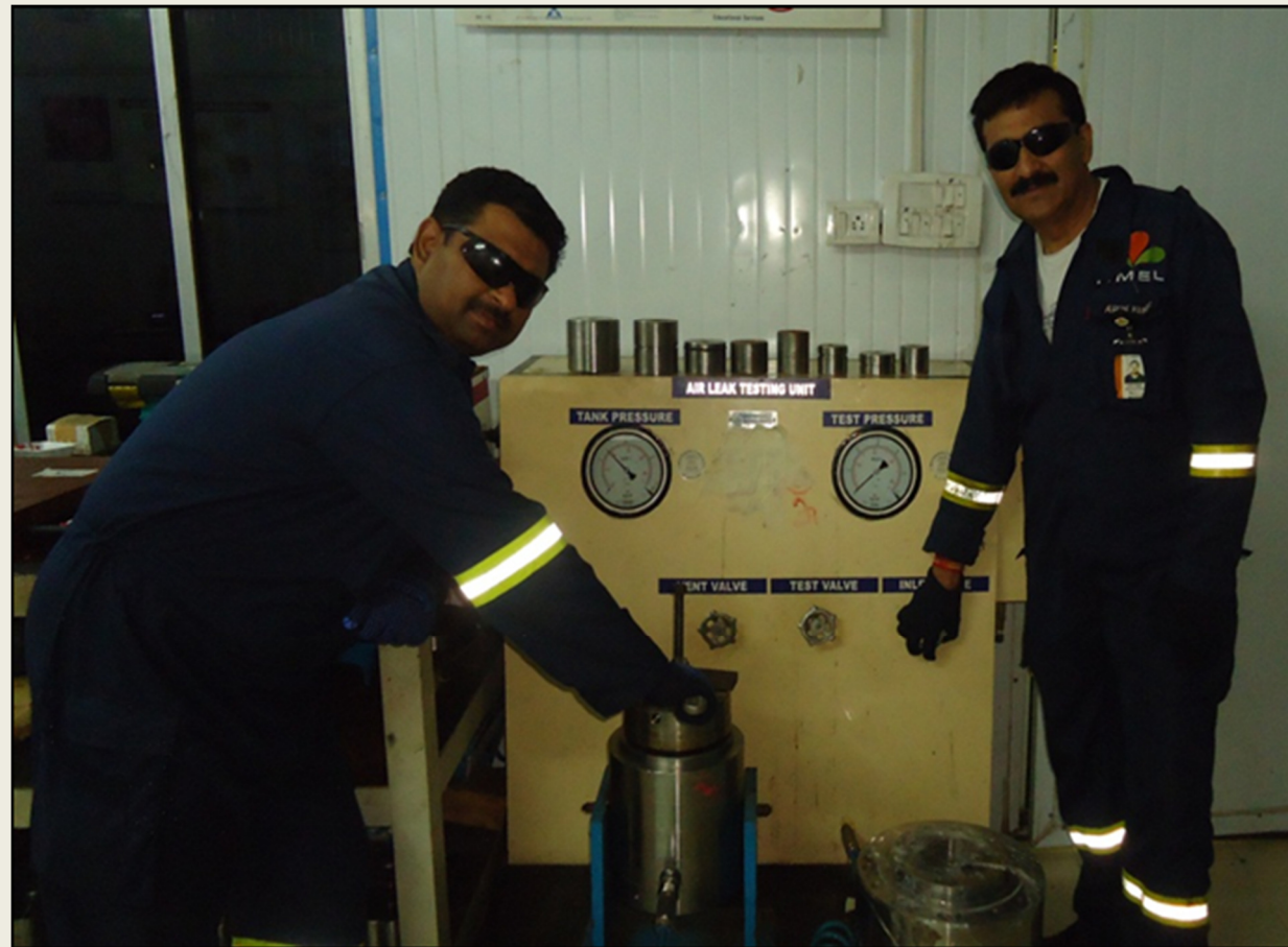
Air Leak Testing Unit
