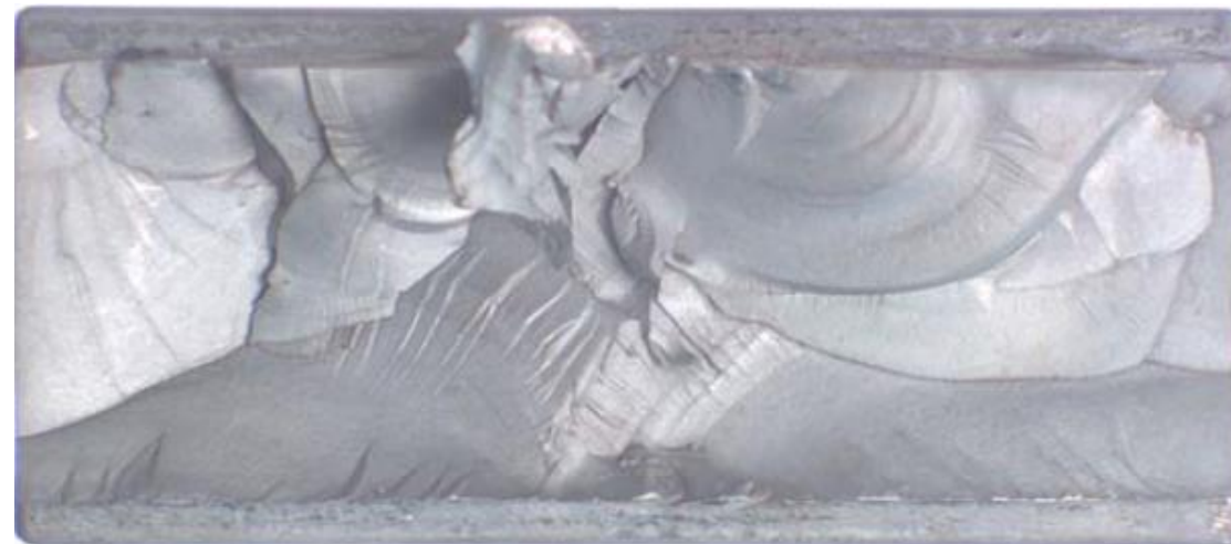
Fig.1 Fracture surface of No.70 blade
