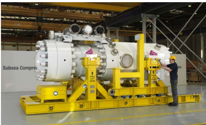
Figure 6: Subsea Motor-Compressor Mounted on its Transportation Frame
