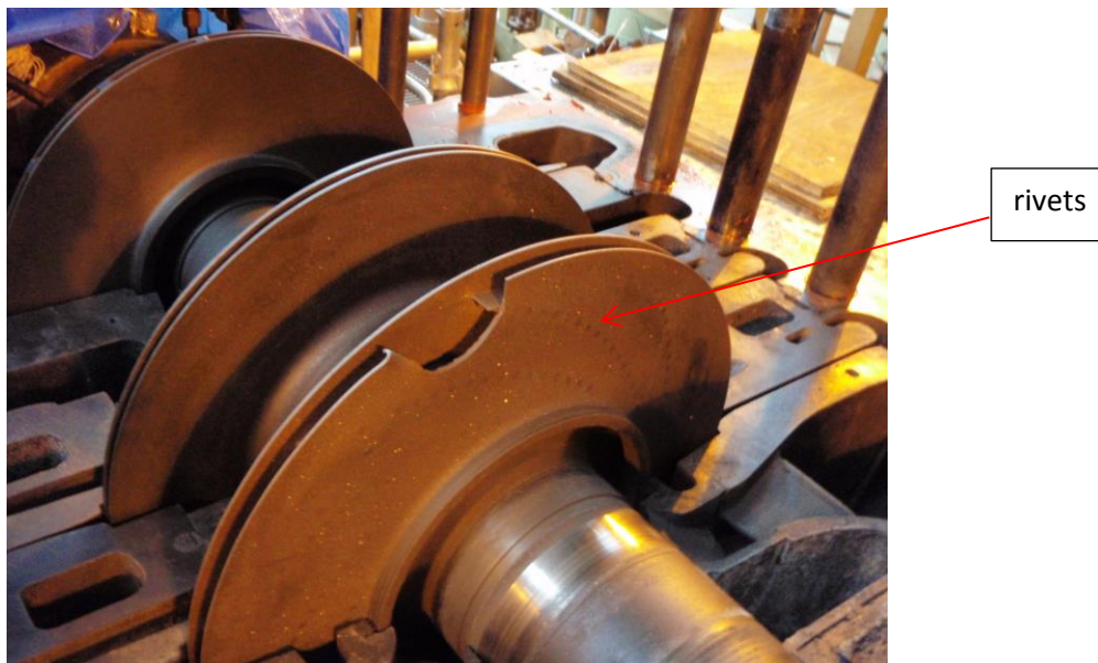
Figure 43. FCC wet gas compressor failed 5 th stage impeller, note rivets
