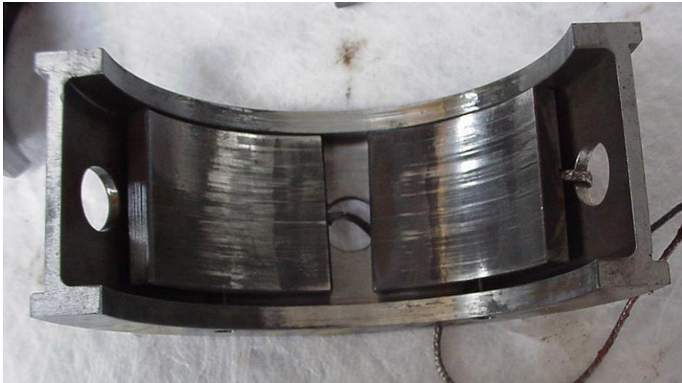
Figure 16. Wiped tilt-pad bearing (due to insufficient lubrication) from reformer recycle hydrogen compressor
