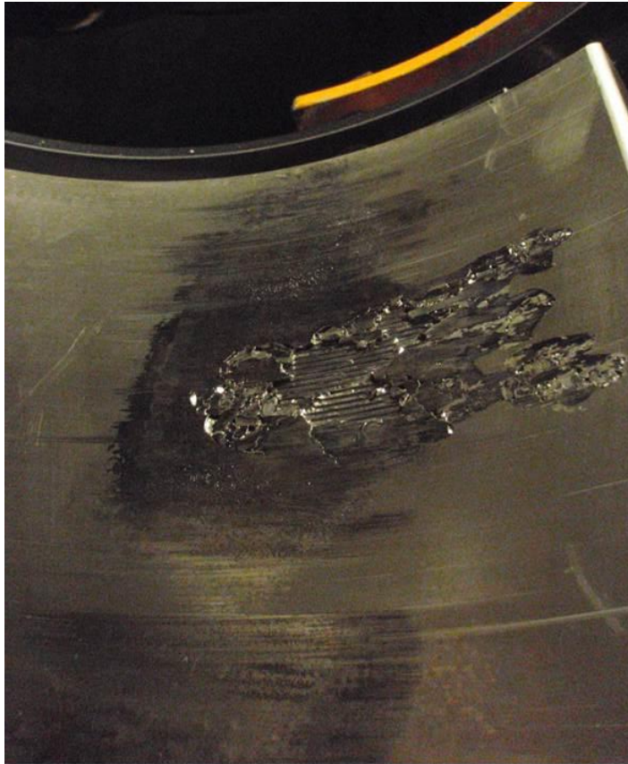
Figure 53. Damaged pad from #3 bearing found during bearing inspection after overhaul
