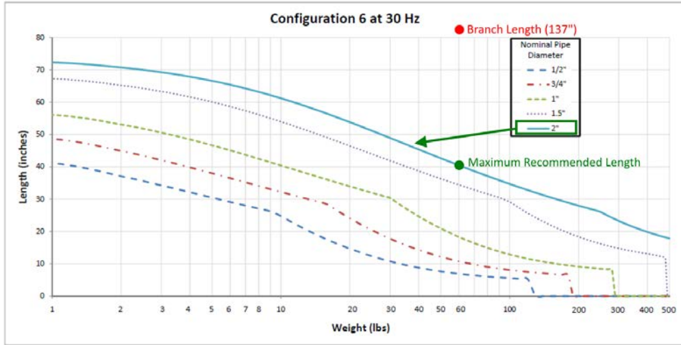
Figure 23. Graph Providing Maximum Span Lengths for Configuration Type 6 from GMRC/PRCI Guideline Using the EI Guideline
