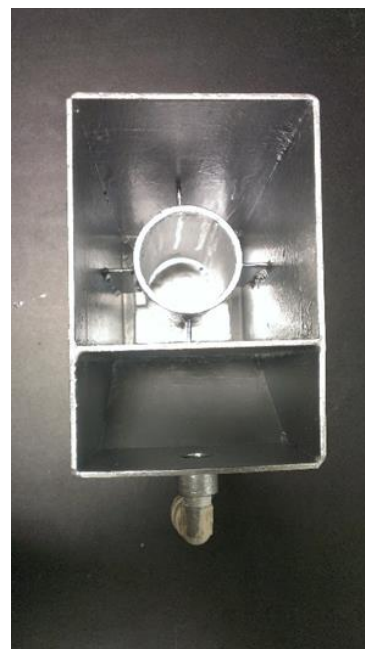
Figure 25. Schematic representation (left) of the flow-through CSTR treatment system (not to scale) and the photo (right) of the reactor with 2 L reaction zone.
