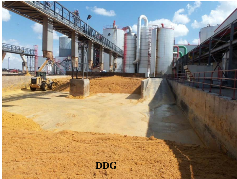
Figure 5. White Energy Inc. biofuel industry in Plainview, Texas. Aflatoxin will be enriched in DDG if contaminated corn is used for ethanol production. Photo was taken by the soil mineralogy group in the department of soil & crop sciences, TAMU.
