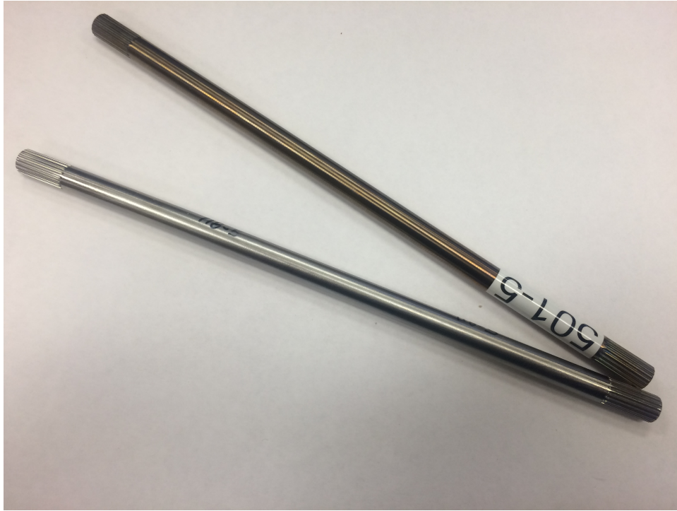
Figure 1.3: 3/8" Nitinol torque tubes used for control experiments.
