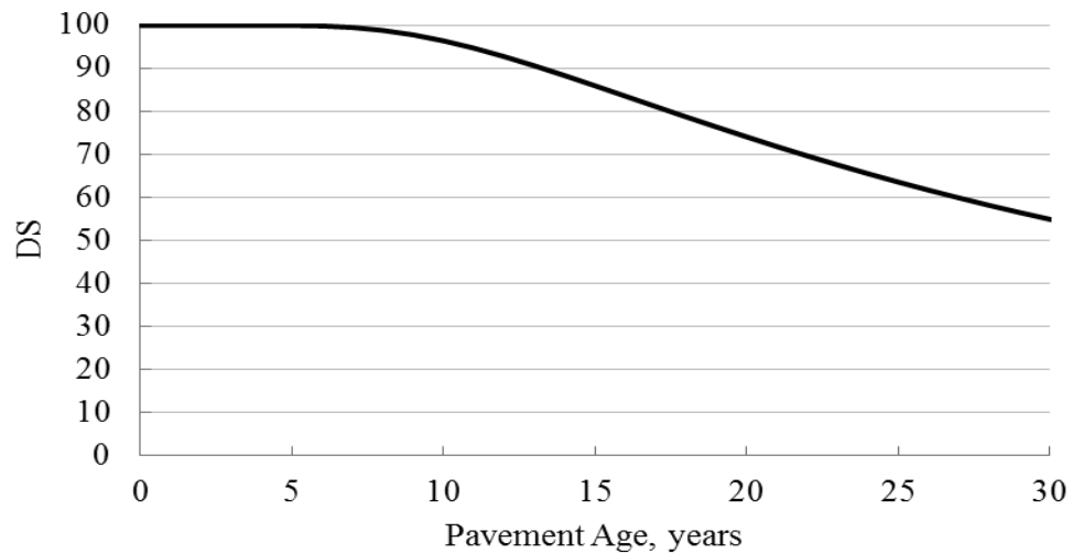
Figure 33 Example DS prediction model (pavement B, Zone 1, medium traffic loading, and LR treatment).
