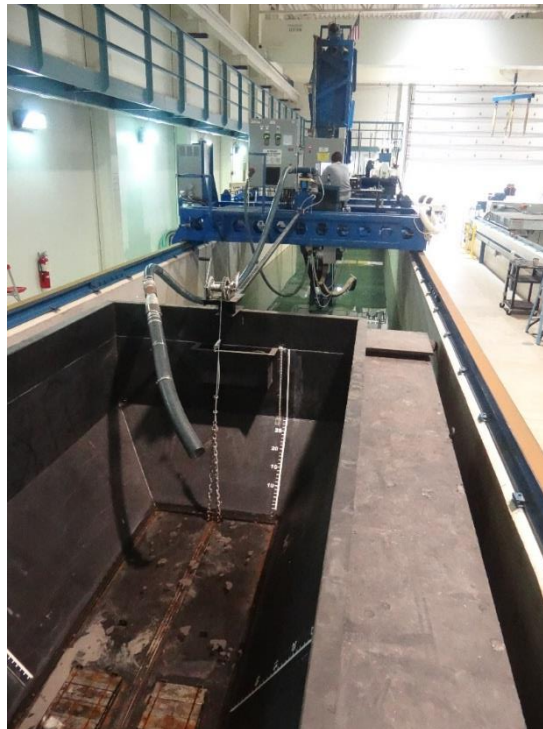
Figure 28: Photo of the carriage connected to the barge in the tow tank.
