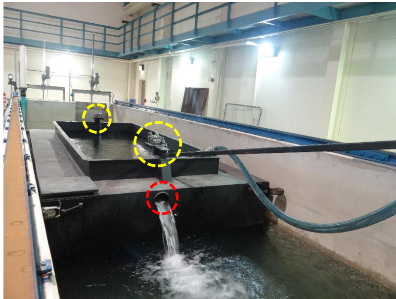
Figure 31: 3 in discharge line into the barge, which is equipped with two winches (yellow) and a weir (red).
