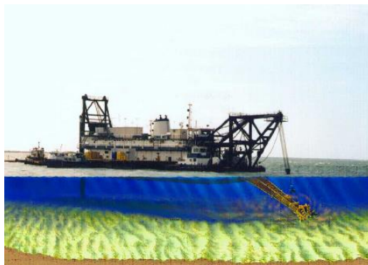
Figure 8: Schematic drawing of a Cutterhead Suction Dredge. Source: US Army Corps of Engineers.
