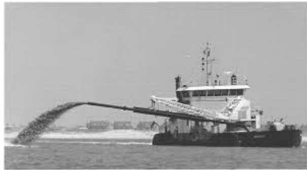
Figure 7: A Sidecasting Dredge in operation. Source: US Army Corps of Engineers.
