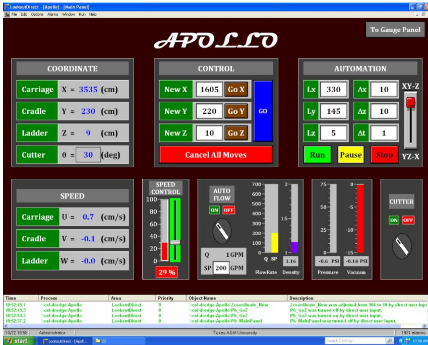
Figure 37: Graphic interface of the software Apollo used to control the cutterhead model dredge.
