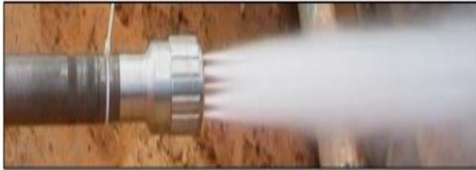
Figure 8: Jetting Nozzle Assembly for Acid Tunneling (Portman, 2002)
