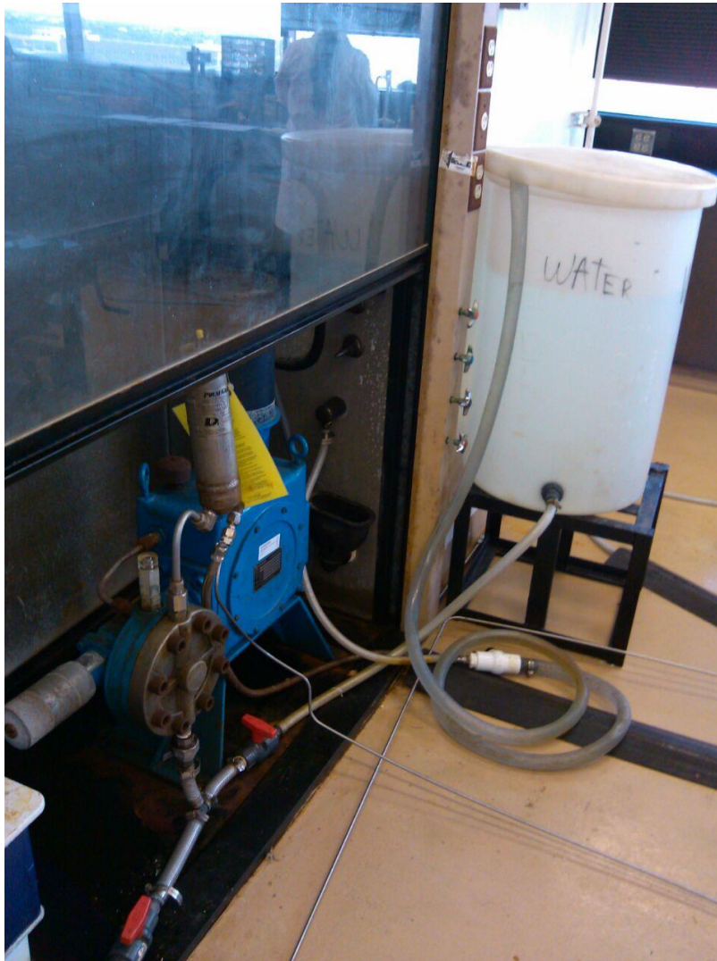
Figure 14: Experimental Setup - Water Tank and Injection Pump
