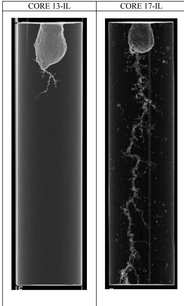
Figure 26: Acid Jetting at Injection Rates of 150 ft/s and 107ft/s for V_i of 0.14cm/min
