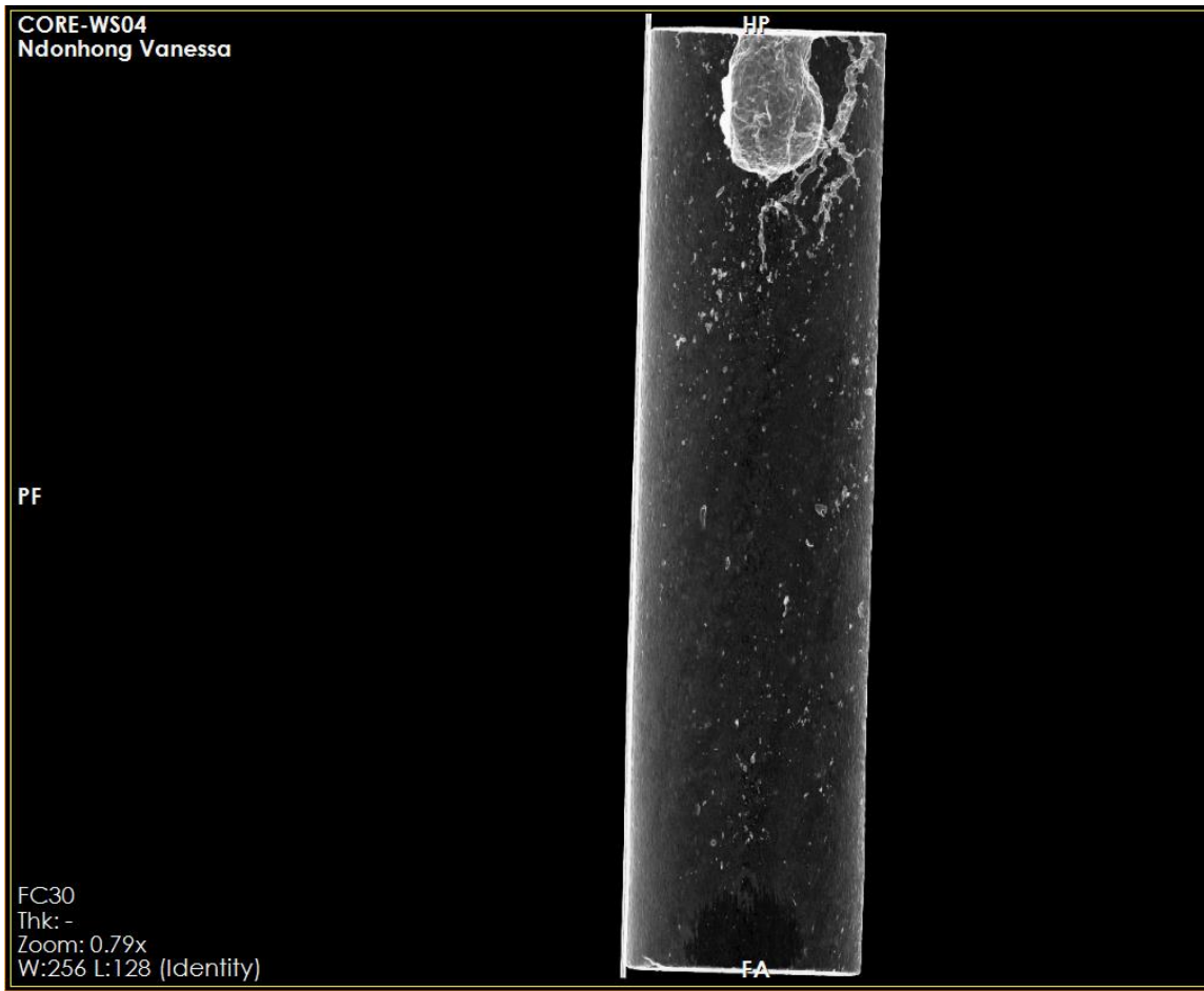
Figure 44: Core WS04 CT Scan after Acid Jetting
